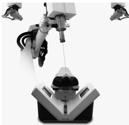
Fig. 1. The CyberKnife radiosurgical system. Note the two amorphous silicon x-ray screens positioned orthogonally to the treatment couch. The couch can move to position the fiducials in front of the cameras.
